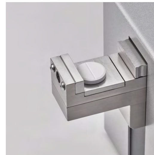
Quick-change tongue with flat surface
