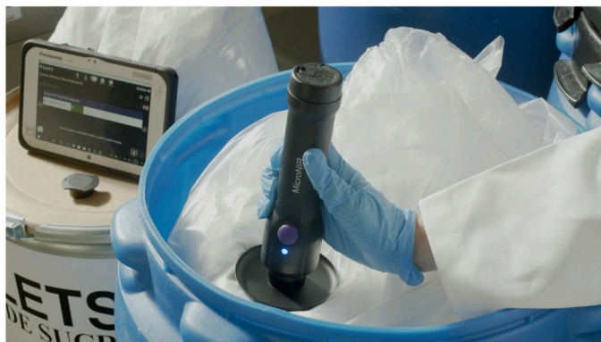
Figure 4. The sampling collar, single push-button operation, rapid measurement cycle, and lightweight of the MicroNIR OnSite-W minimize sampling errors and fatigue. Results are displayed rapidly on the Bluetooth-connected tablet PC.
