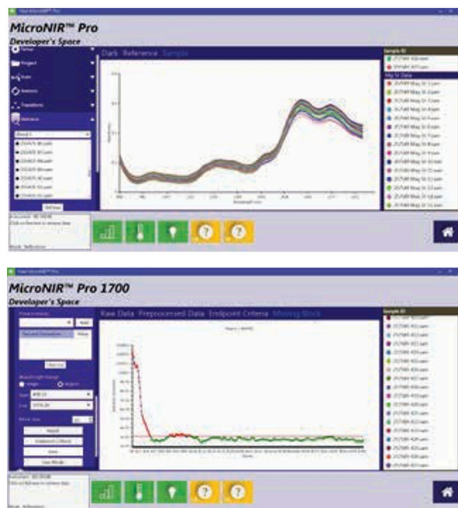
Figure 3. a) Spectra acquired during blending. b) Moving Block Standard Deviation of spectra plotted over time.
